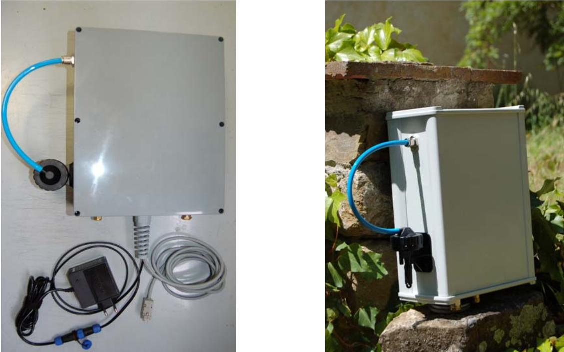
Fig.2 Indoor (left) and Outdoor (right) versions of the LCT-12 measuring station. PM measuring stations can be integrated with NDIR or electrochemical trace gas sensors, to monitor other possible pollutant.
