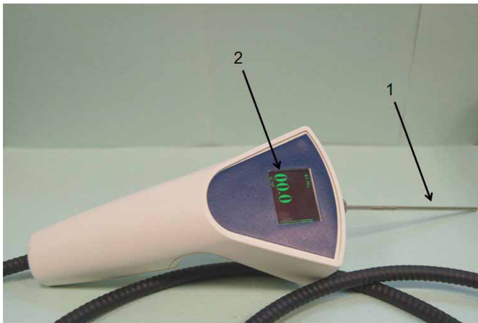
Figure III.3: 1) Stainless steel capillary , 2) OLED color screen.
