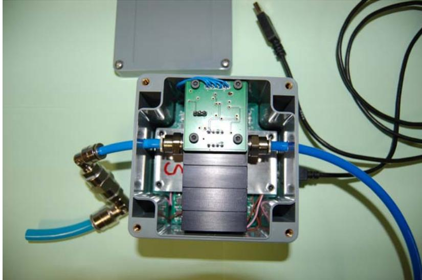
The 10 x 10 x 9 cm ABS protection BOX contains the Laser-scattering cell and the electronics devoted to the processing of the optical signal.
