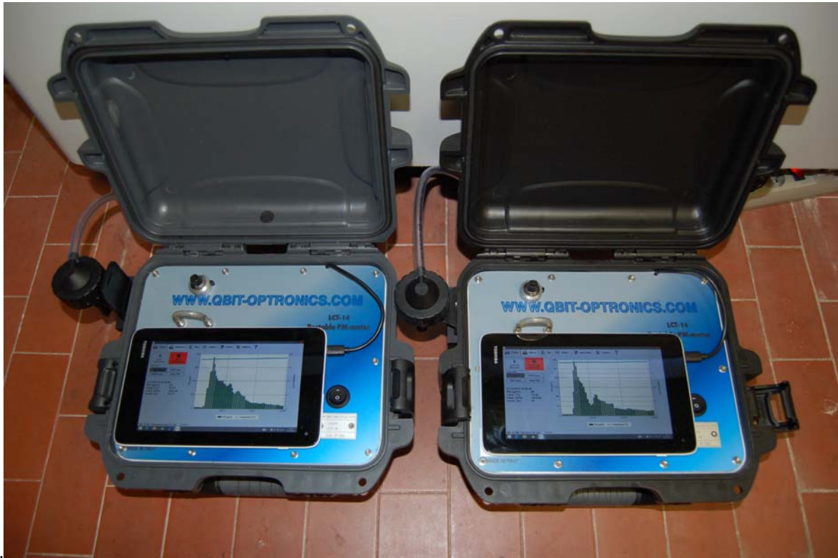
Figure III.1. Main panel. In this figure are shown two main units in standard configuration, with cyclone filter and Toshiba Encore Mini WT7-C-100 tablet.
