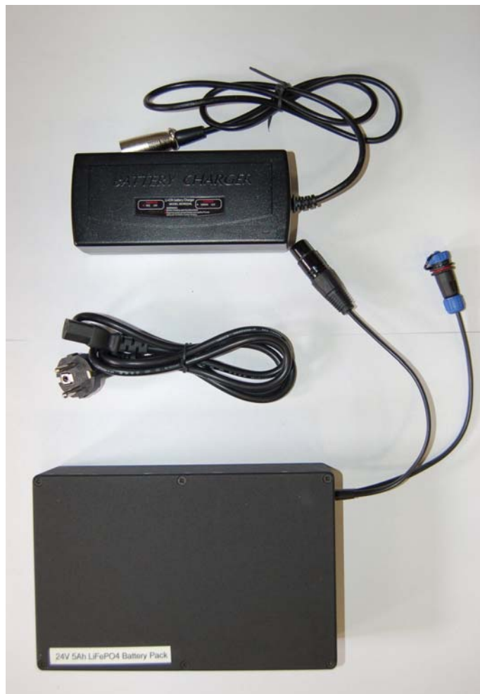
Figure III.4. Battery and battery charger.
