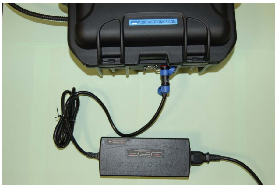
Figure V.1. Connection to AC line.
