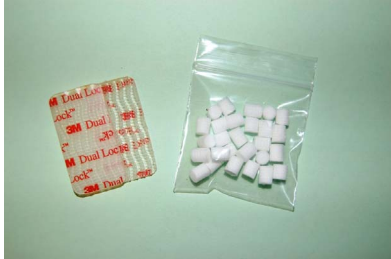
Figure III.5: Tip filters for sniffer and self-adhesive Velcro strips.
