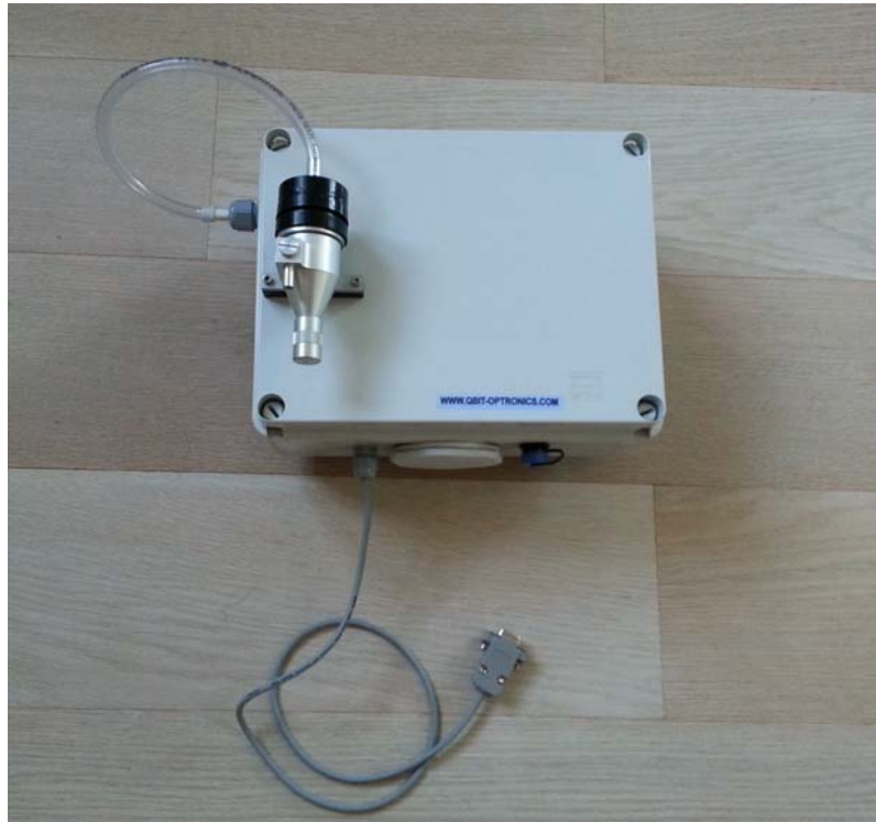
Figure III.1. Main unit. In this figure is shown the LCT-12N in standard configuration, with PM10 cyclone filter and RS232 interface.
