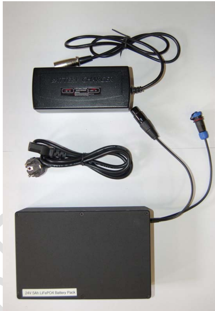
Figure III.4. Battery and battery charger.
