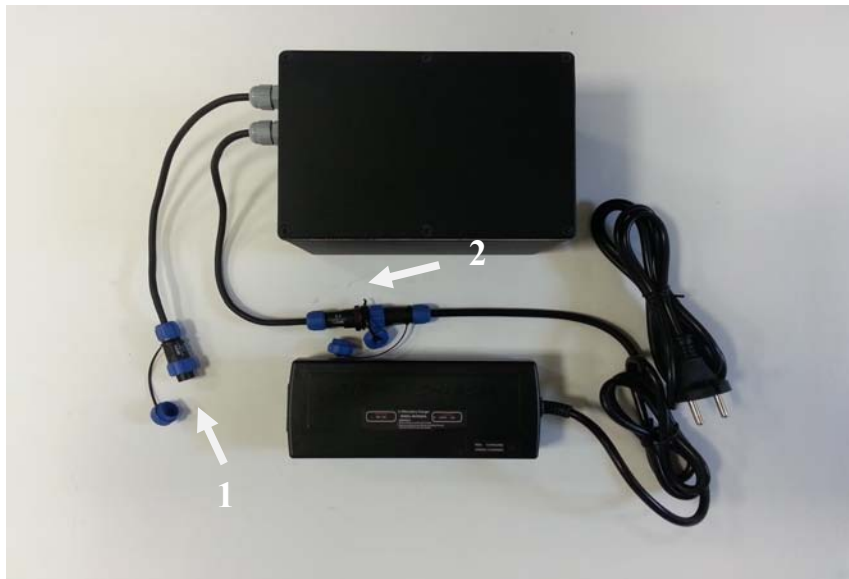
Figure III.7 External battery. 1) LCT-14 plug. 2) Battery-to-charger connector.
