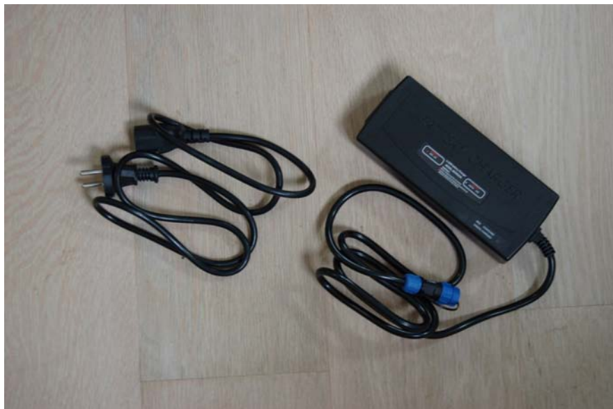
Figure III.6 Power supply / battery charger.
