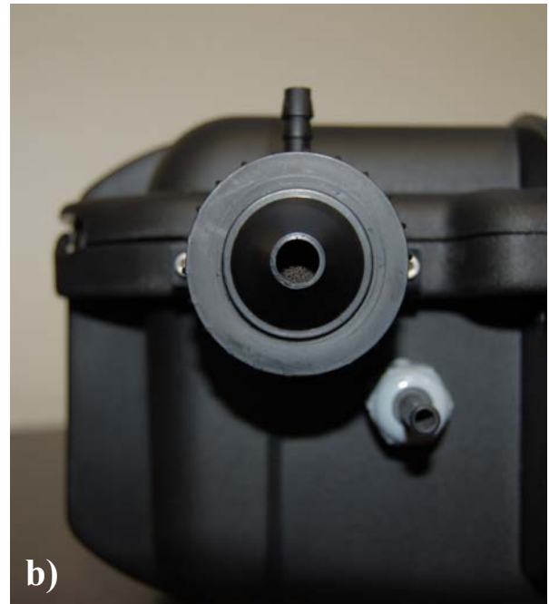
Figure III.5. PM selectors. a) PM2.5 cyclone filter. b) PM10 porous filter.
