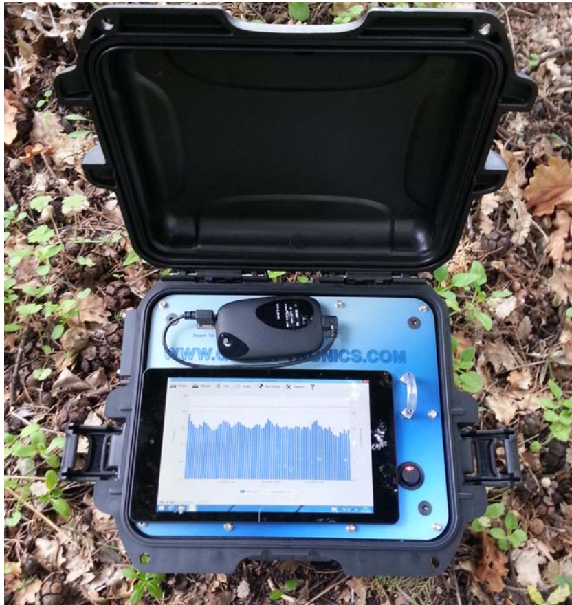
Figure III.8. External wireless router.
