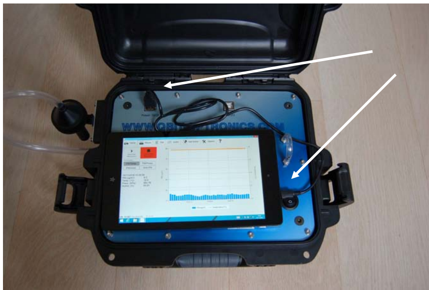
Figure III.3 USB-A connection. The external control unit, connected and powered via USB-A, remains working with the instrument. In this way, working time is not limited by the internal battery if the main unit is connected to 220VAC line.
