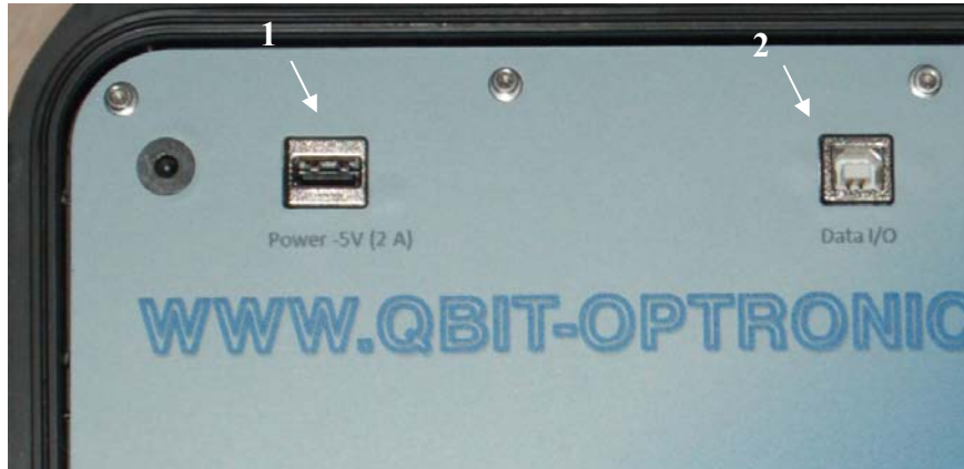
Figure III.2 Main panel USB plugs: 1) USB-A [Power 5V-2A] and 2) USB-B [data]
