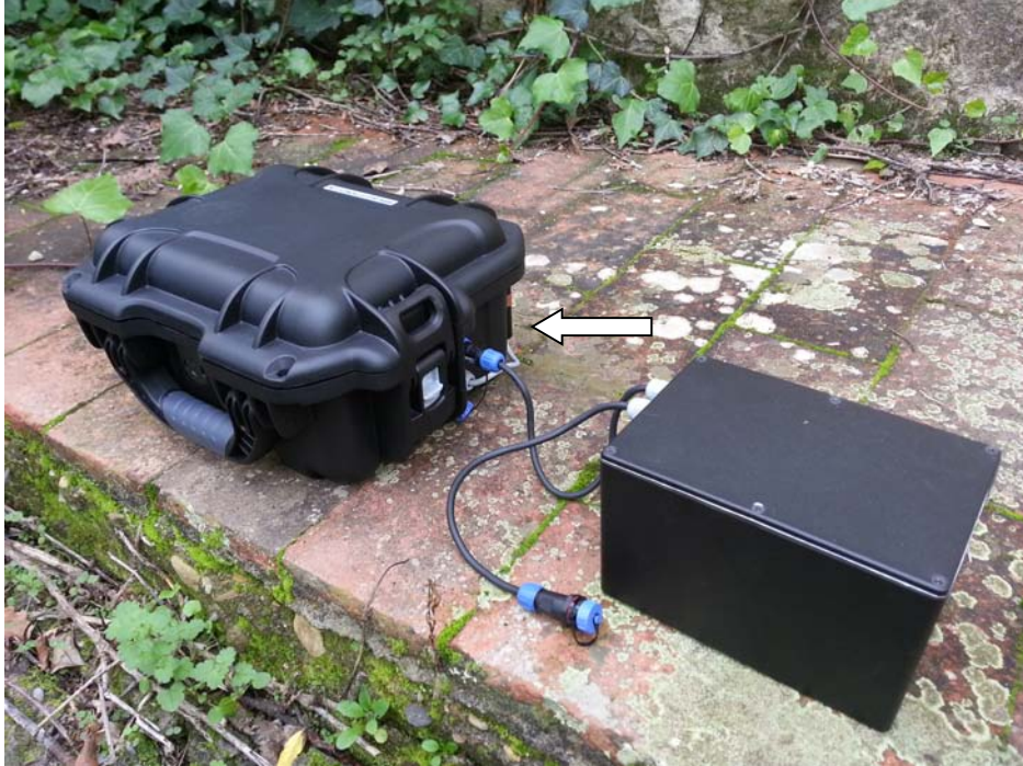
Figure V.4. Connection to external battery.
