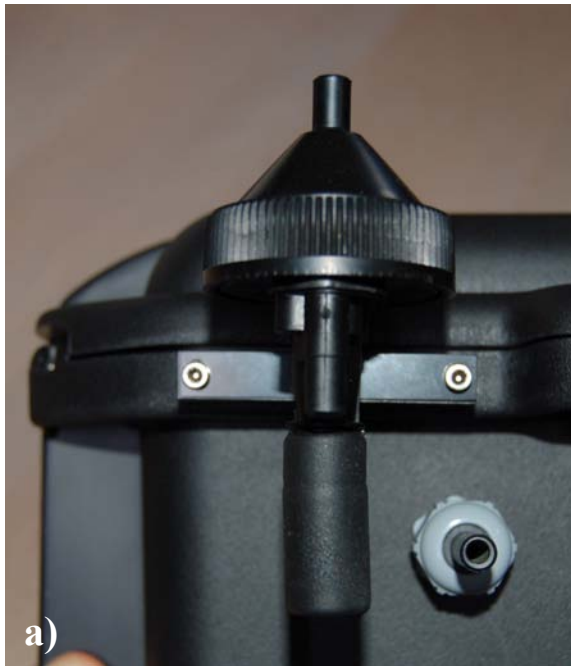
Figure III.5. PM selectors. a) PM2.5 cyclone filter. b) PM10 porous filter.
