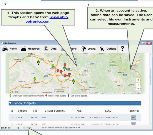
3. The internet connection is shown here. When orange, the instrument is uploading data to the server (files are uploaded every 10 minutes when the automatic procedure is selected). If a measurement is running, the corresponding file will be uploaded later or when the file dimension reaches 1Mbyte.
